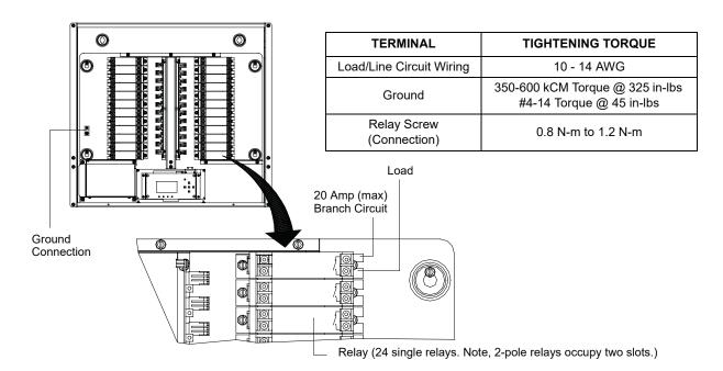
FIGURE 4. LINE/LOAD WIRING CONNECTIONS
