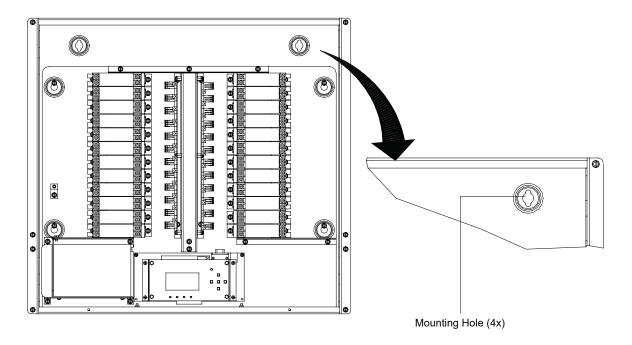
FIGURE 3. PANEL MOUNTING HOLES
